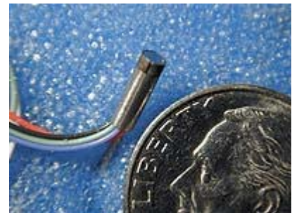
The miniature piezoresistive semiconductor pressure transducer is targeted for applications such as unsteady flow measurement in wind tunnel model testing of the Joint Strike Fighter.
