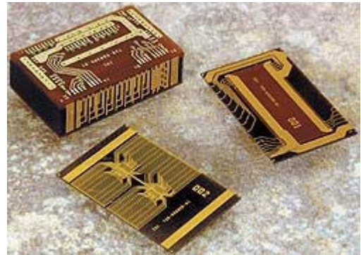
The NeoStack from Irvine Sensors is a microsensor based on chip-stacking technology and integrates support electronics with the sensors, rather than packaging support electronics in separate boxes.
